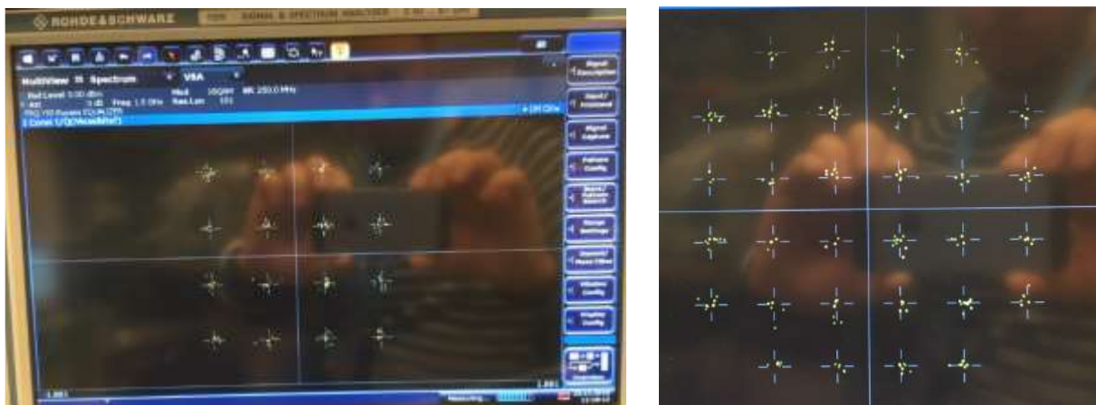
Figure 9: Screenshot of the constellation diagram for 16 QAM and 32 QAM observed for the Tx3-Rx2 link
